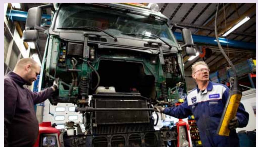
FIGURE 3 - NOW IT'S TIME FOR LIFT-OFF. JIMMY GUSTAVSSON (LEFT) AND KENNETH OLSSON (RIGHT), GUIDE THE CAB TO ENSURE IT DOES NOT STRIKE AGAINST AND DAMAGE THE RADIATOR AND ENGINE.
