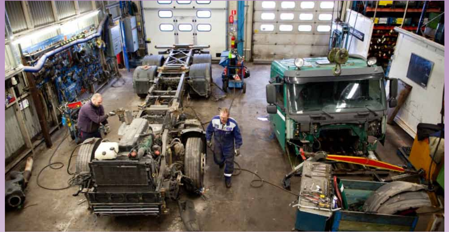
FIGURE 4 - ONCE WIRES, HOSES AND PIPES, NIPPLES, CLAMPS AND CLIPS HAVE BEEN REMOVED, IT'S TIME TO LIFT OUT THE GEARBOX AND ENGINE. LAST OUT ARE THE BEAMS, AXLES AND BRAKE CALLIPERS.
