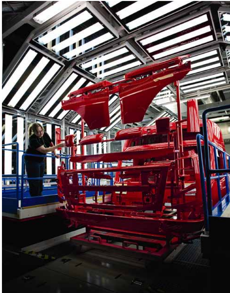
FIGURE 3: MOST OF THE WORK AT THE FACTORY IN UMEÅ IS AUTOMATED AND HANDLED BY ROBOTS. HOWEVER, AFTER THE TOPCOAT HAS BEEN APPLIED, EVERY CAB IS CHECKED MANUALLY TO ENSURE THAT THERE IS NO DAMAGE, NO SCRATCHES OR UNEVEN PAINT APPLICATION.
