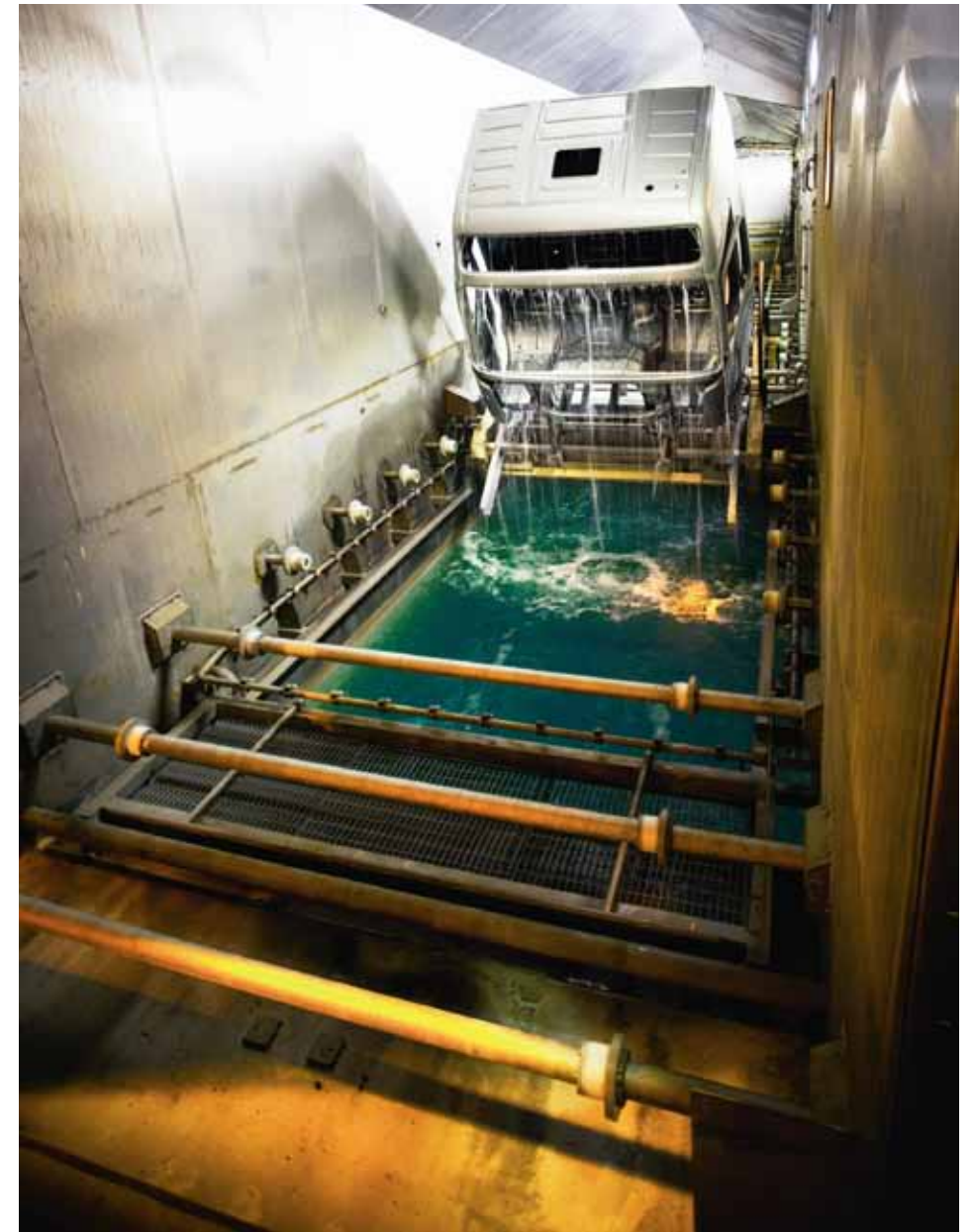
FIGURE 2: PRE-TREATMENT. THIS IS ONE OF THE “CHEMICAL BATHS” IN THE PROCESS, WHICH ENSURES THAT THE METAL IS TOTALLY CLEAN SO THE PAINT CAN ADHERE PROPERLY.
