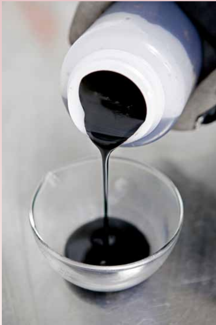
FIGURE 3: BLACK LIQUOR IS A BY-PRODUCT THAT IS “LEFT OVER” WHEN THE CHIPS ARE BOILED.
