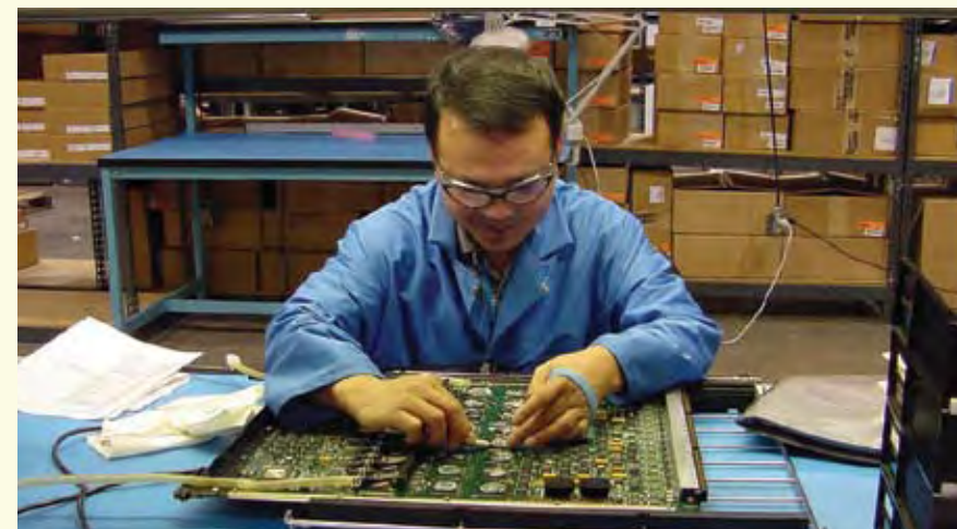
Sr. Technician reworking and troubleshooting water-cooled PCA
