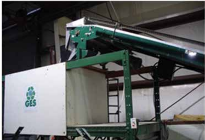
CRT Crusher – Crushed CRT glass is conveyed in the “Crusher”
