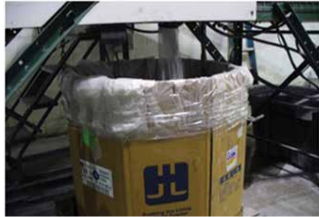
CRT Sand – Crushed CRT Sand comes out of the “Crusher”
