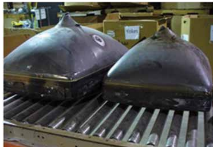
CRT Line – CRTs are sent down a conveyor to begin the process
