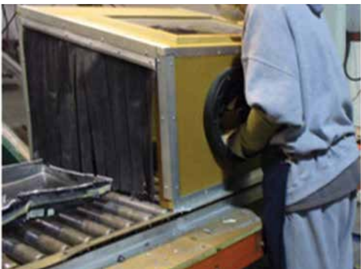
CRT Crushing Box – CRT Glass is crushed into smaller pieces
