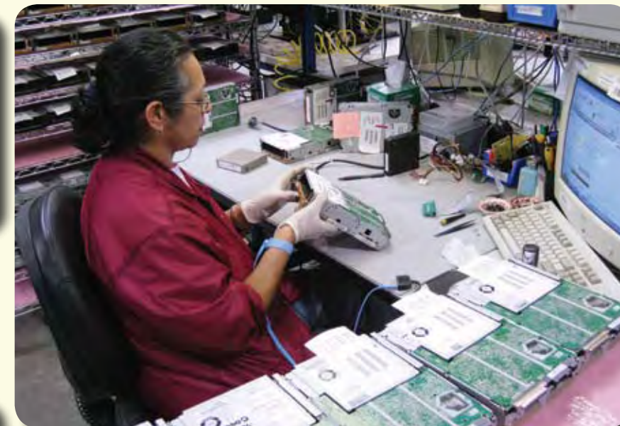
Dominga Castro thoroughly inspects units for physical damage and missing parts prior to being routed to the appropriate process station.
